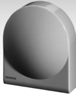
QAC Outside Sensor Operable at the range of -50°C to 70°C. Allows connection at maximum 120 meters using cable with 1.5 mm 2 section
