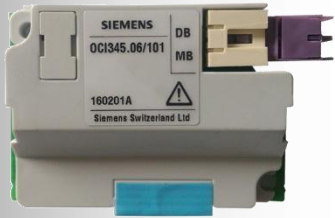
OCI345.06 CASCADE Module For wall mounted boilers, 16 boilers, including 1 master and 15 slave boilers, can be controlled as cascade
